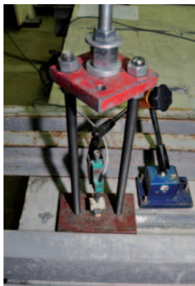
Test setup for cyclic pull out tests
