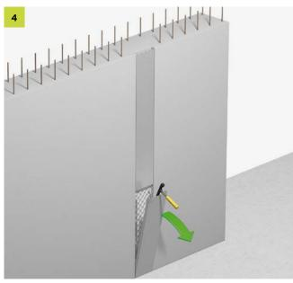
After the first concreted section, remove the covers and the polystyrene stopper strips at the ends.
