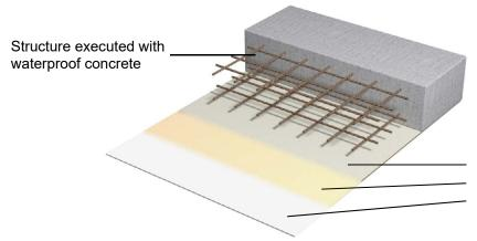
Fully bonded, pre-applied flexible sheet for waterproofing "SECUFLEX SMT 1212" with a three-layer structure consists of:
