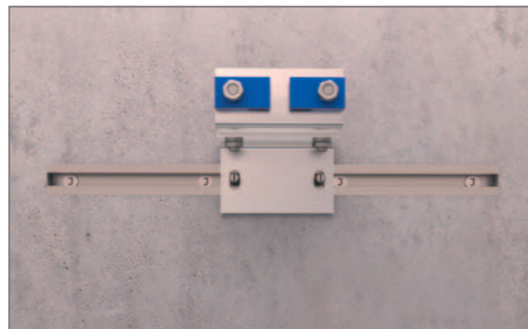
After installation, check the correct seating of the T-bolt in the anchor channel – the marking slot must be perpendicular to the channel axis.
